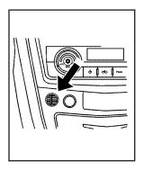
There is also an interior temperature sensor located below the climate control system next to the steering wheel.
